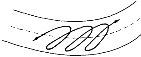
Fig 7.3 Toroidal precession of a banana orbit.
